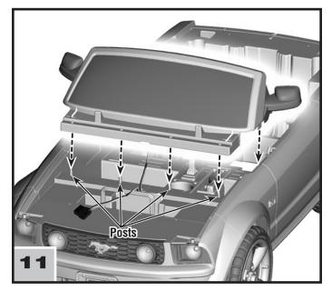
• Fit the dash assembly onto the posts near the front end of the vehicle.
